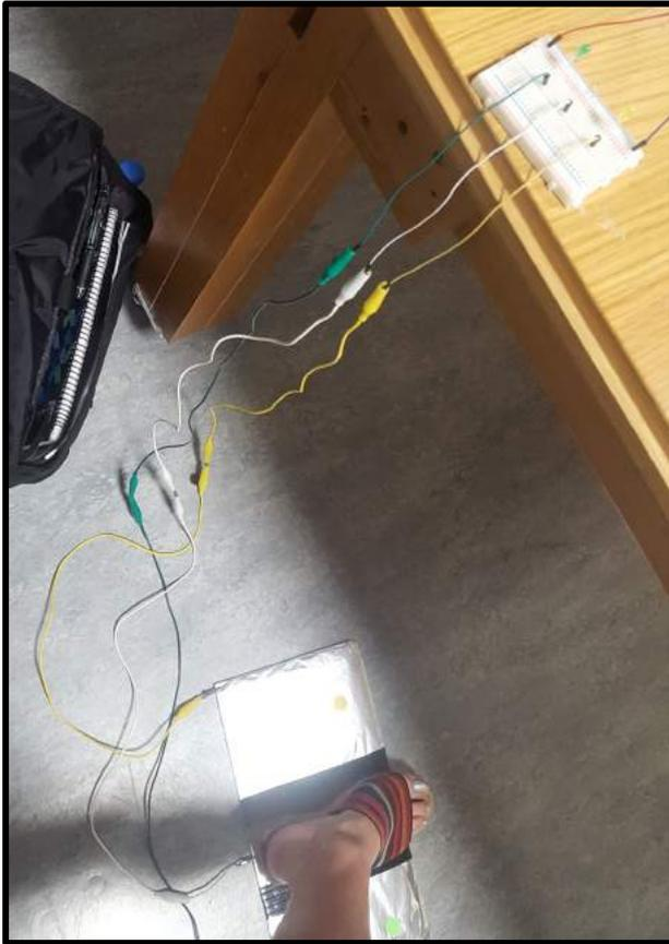
Thus, the pedal works as follows: when an individual's foot is facing forward, no lights turn on. However, if the foot is angled to the left (towards the yellow dot/wire), the yellow LED light turns on. If the foot is angled to the right (towards the green dot/wire), the green LED light turns on.
